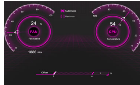
Figure 8 - Fan Speed Control
